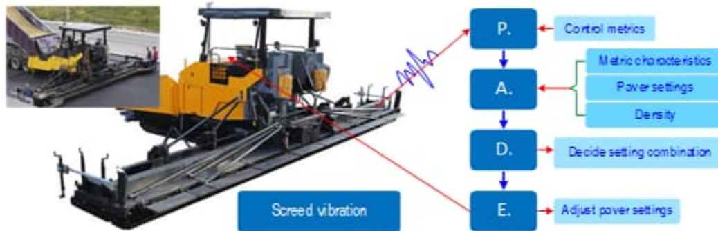
Figure 4: Feedback Control for Enhancing Paving Quality
