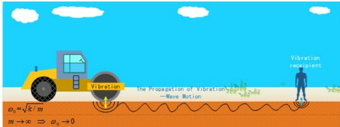
Figure 3: Wave Phenomena Generated by Vibratory Rolling
