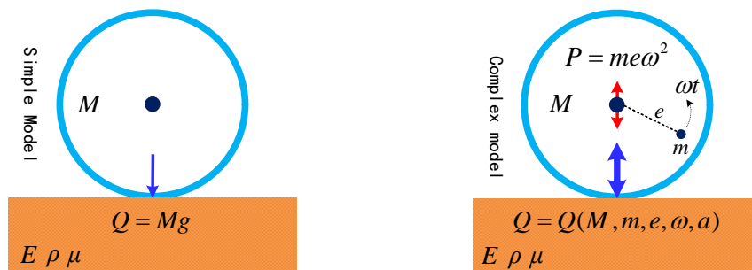
Figure 1: Vibratory Compaction Force vs. Static Compaction Force
